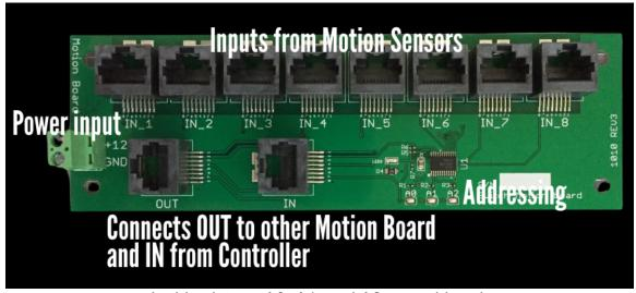
In this picture, A0, A1, and A2 are soldered. Therefore, it is addressed as Switch MOTION Board 2.
