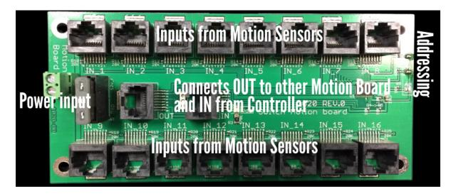
In this picture, A0, A1, and A2 are soldered. Therefore, it is addressed as Switch MOTION Board 2.
