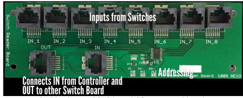
In this picture, A0, A1, and A2 are not soldered. Therefore, it is addressed as Switch Reader Board 1.
